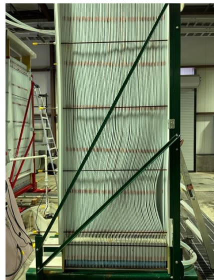
Figure 4 – Failure Mode for Plate Assemblies
