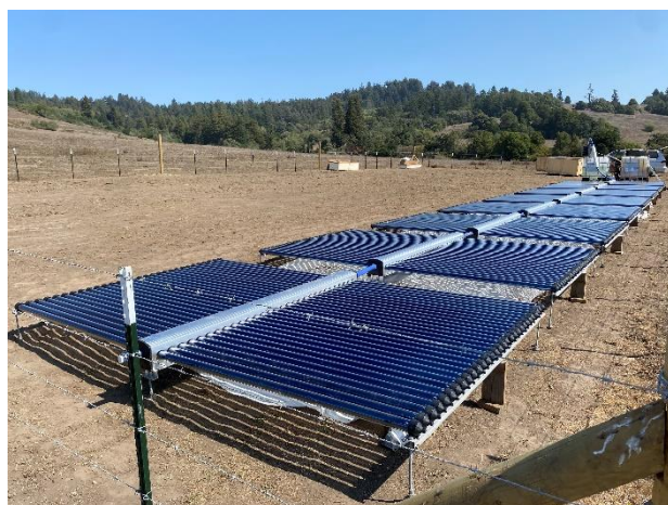
Figure 6 – Eight Panel Array of AILR Steam-Generating Solar Collectors
