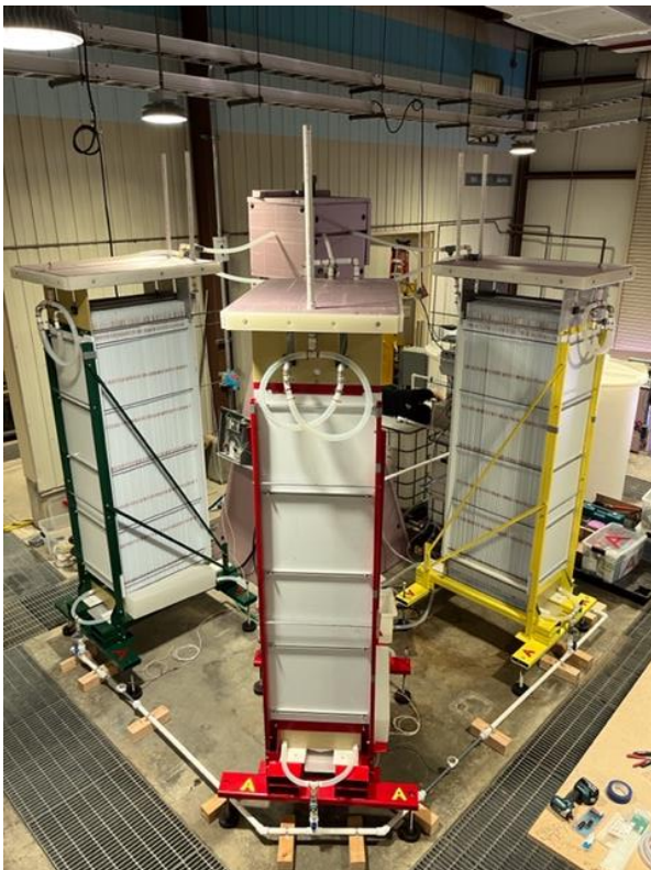
Figure 3 – Three Uninsulated, 70-plate Modules for Brine Zero
