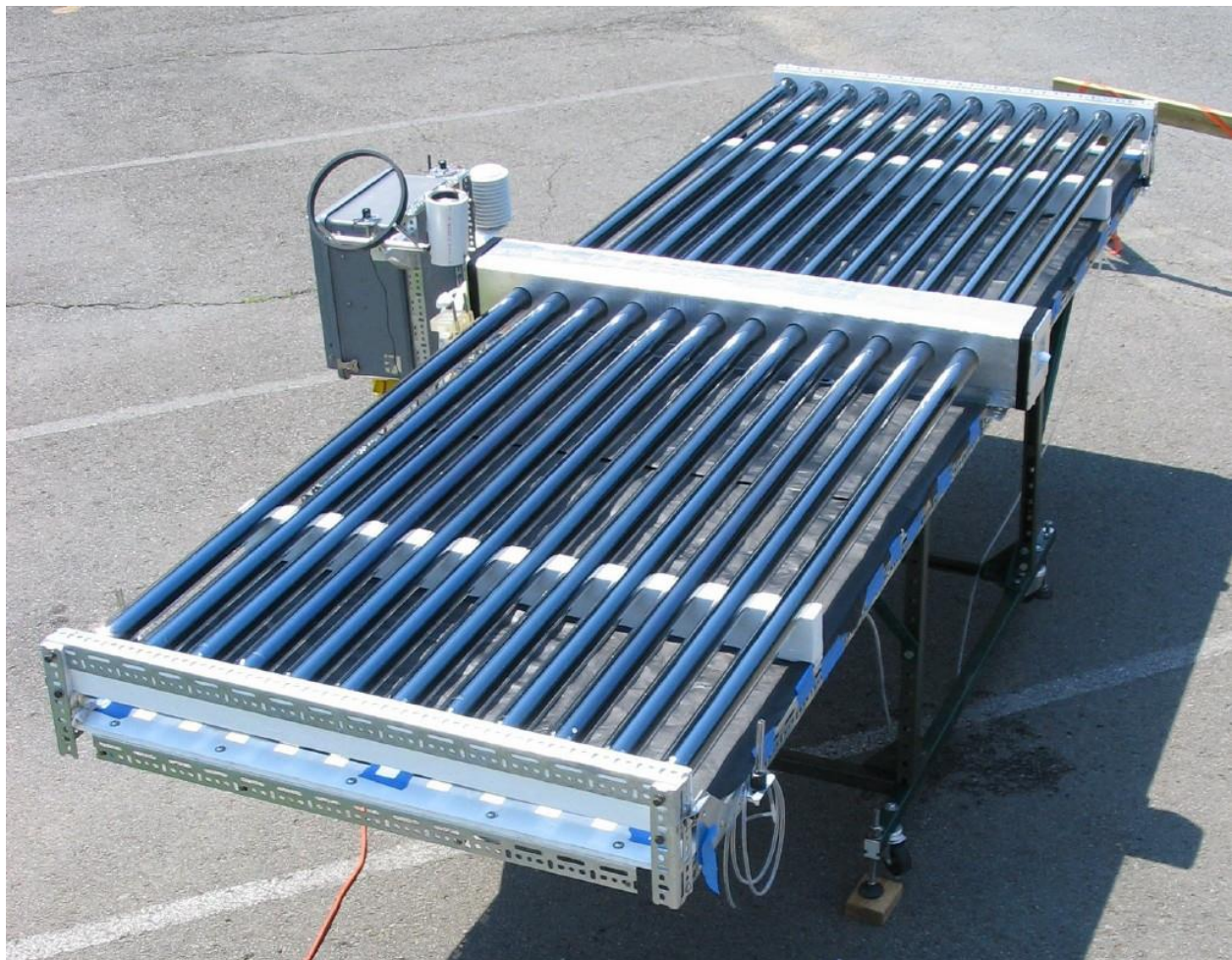
Figure 2. 24-tube collector used for direct steam generation, during testing in 2008.
