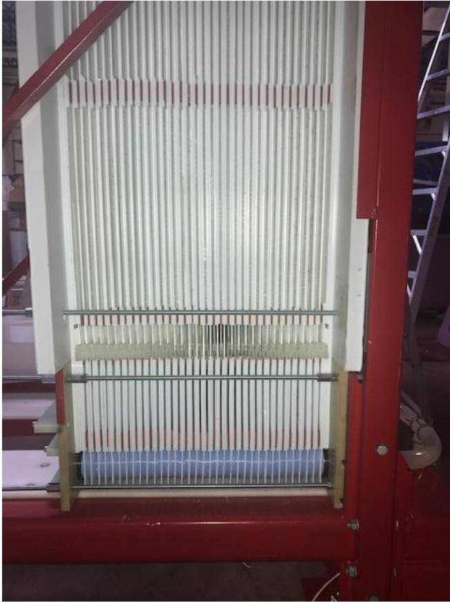
Figure 7 – Retrofit of Red Stack with Continuous Edge Spacers Inserted between the Silicone-Rubber Spacers
