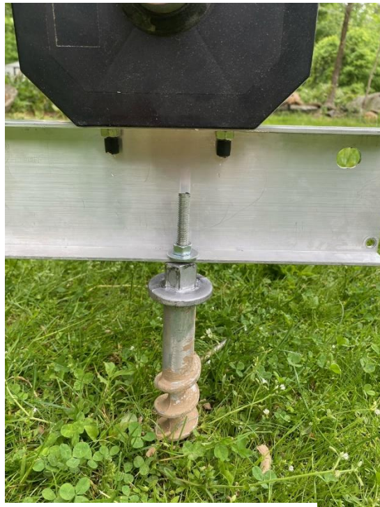
Figure 9 – Array Mounting System Based on Earth Anchors
