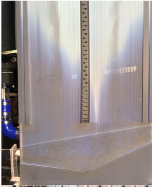
Figure 28 – Flow Non-Uniformity within A Condensing Plate
