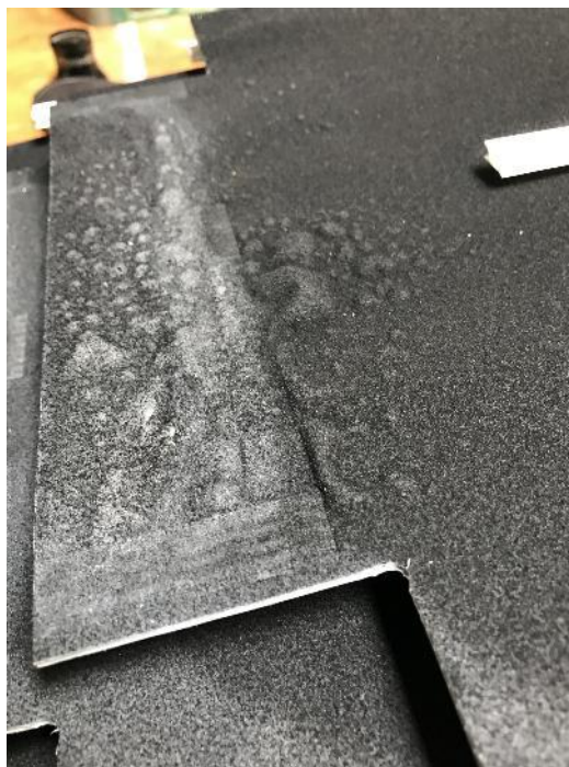
Figure 22 – Bubbling of the Flock Layer
