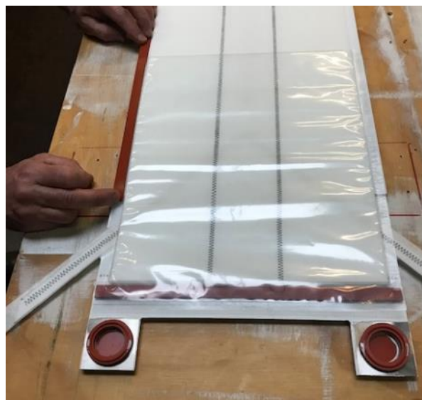
Figure 23 – Design 9 Condensate Collection and Brine/Condensate Isolation
