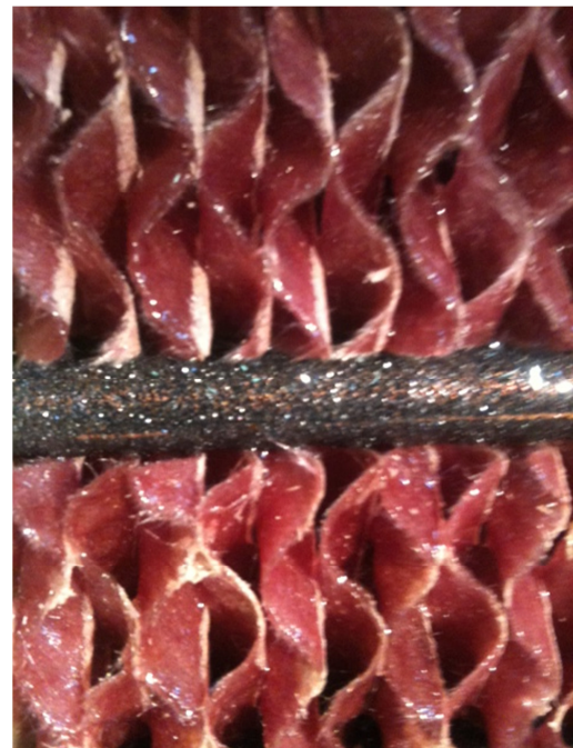
Figure 2 – Wicking Fins Implemented with Corrugated Media
